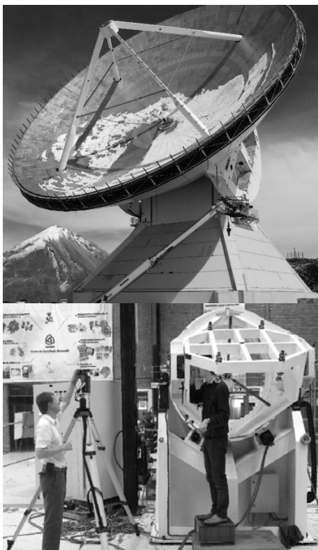
Figure 1. Top: The Large Millimetre Telescope. Bottom: Alignment tests with the tertiary mirror.
