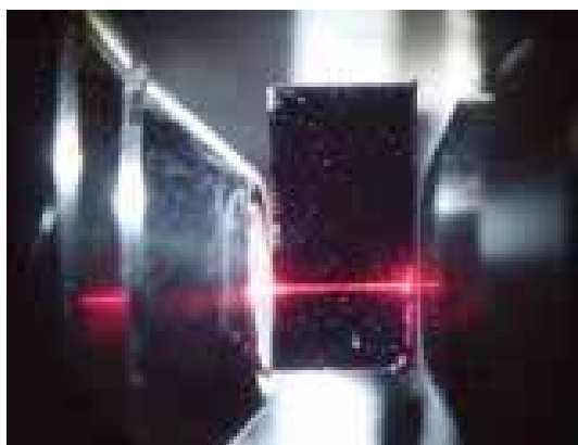
Fig. 2. Light waveguide in a PDLC planar waveguide.
