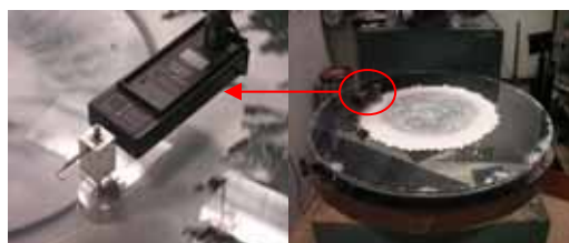
Figure 1: Force sensor holding Teflon® Tool over the workpiece glass.
